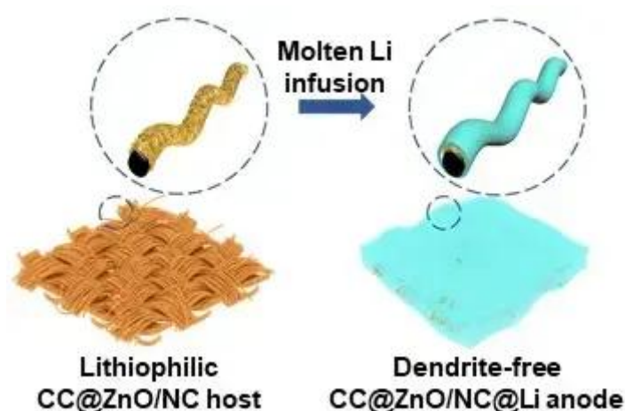
Figure 2. General construction of lithophilic 3D skeleton for dendrite-free lithium metal anode via a versatile MOF-derived route [21].
