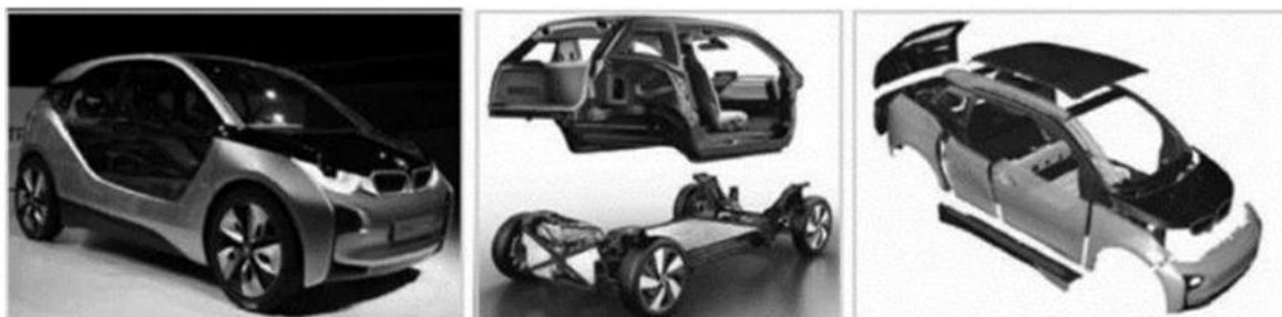
Figure 2. BMW was the first mass-produced light vehicle, and the main parts of its body structure were made of carbon fibre reinforced composite materials [7]
